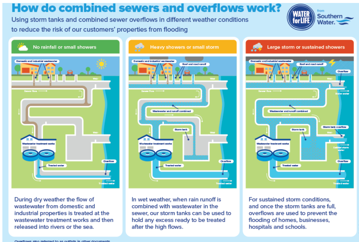
Figure 18 – How combined sewers and overflows work
